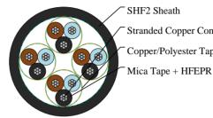
Stranded Copper Conductor Copper/Polyester Tape + Drain Wire Mica Tape + HFEPR Insulation
